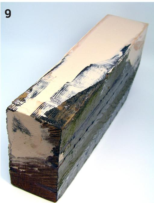
Same repair state as Photo 8. Note the line of holes that have been drilled along the crack. These were sized such that the mixer tip of a cartridge of SilverTip GelMagic adhesive could be seated in the hole allowing GelMagic to be injected into the crack. This both sealed the crack and bonded the two sides together. At this point all the strength has been returned to the beam.
