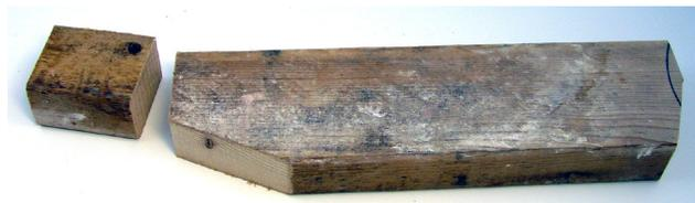
The plywood set into the cavity. These cheap boards replace the volumetrically more expensive SculpWood Putty. Here they are dry-fitted. Note that they lie below the top surface by about 1/4 inch. The boards will be removed and a layer of SculpWood putty will be applied to the bottom. The boards will be shoved into this and the putty pushed into the cavity between the board sides and the putty applied in Photo 4. The putty will fill the two cavities to about the top of the boards.
