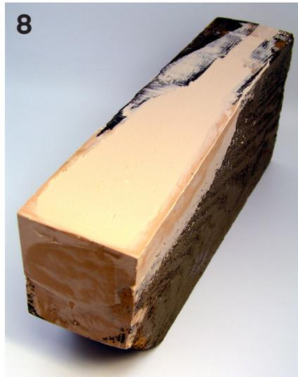
The slight recess in the top has been filled with SculpWood Paste using the newly formed edges as a guide. The side edges have been faired in.
